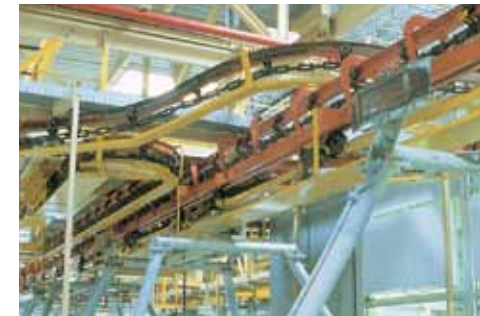
Chains exposed to ambient media, such as in this overhead conveyor in the automotive industry
